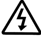
Danger!: High Voltage
